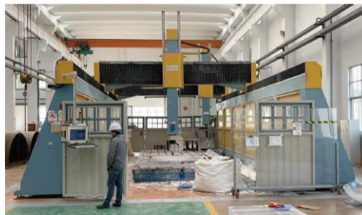
5-axis CNC selected for the TPC barrel machining
